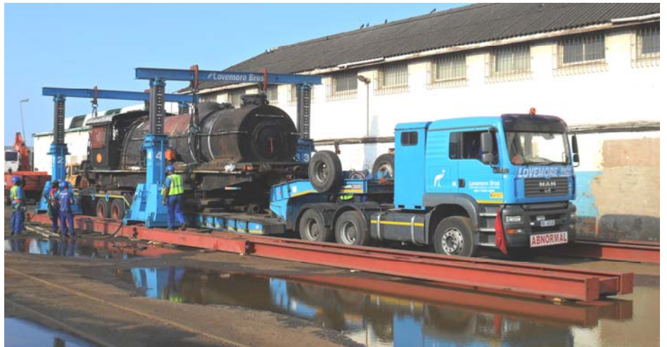
On arrival at Maydon Wharf the locomotive is offloaded using gantries to raise her
