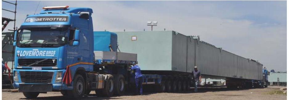
One of the pontoons makes its cumbersome way from the point of fabrication to the wharf. Note the 'push-pull' method of transportation using two trailers
